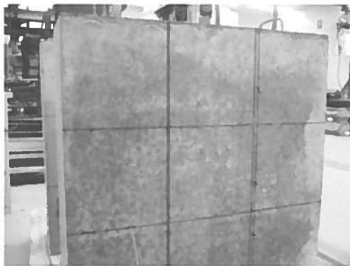
Figure 4: CPF concrete block after demoulding.
