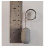
An individually connected sacrificial anode which acts to prevent corrosion initiation in reinforced concrete structures.
