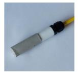
A long life pseudo reference electrode used to measure steel potentials in reinforced concrete
